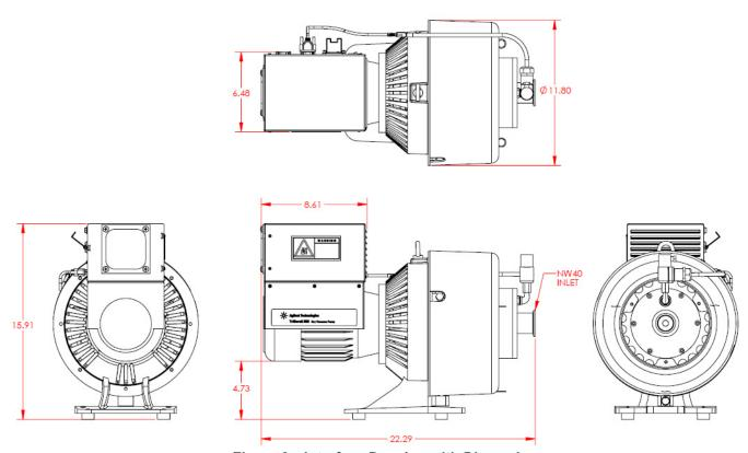
Figure 2 Interface Drawing with Dimensions
