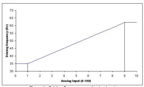
Figure 4 Driving Frequency vs. Analog Input
