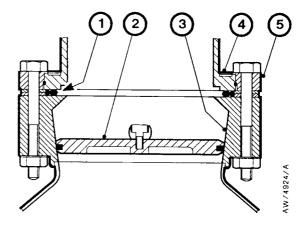
Figure 10 - F-model Diffstak inlet connection
