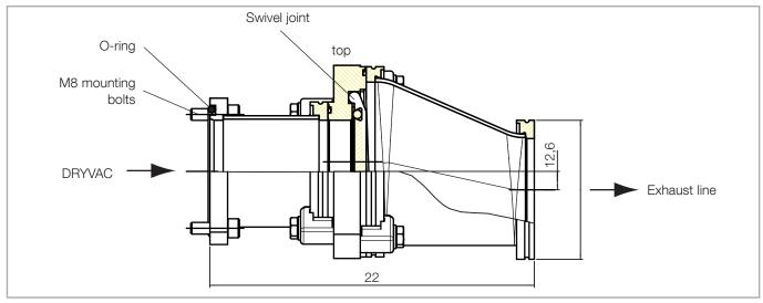
Fig. 3.23 Side view/sectional view of the non-return valve
