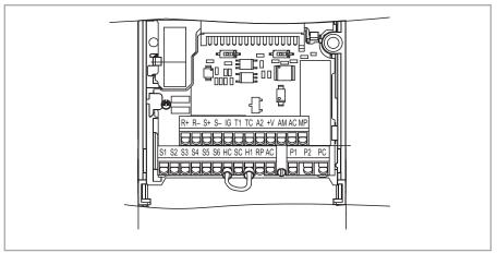
Fig. 3.14 Control circuit terminals
