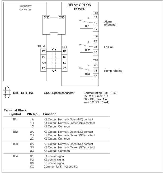
Fig. 4.3 Relay option board: Connections
