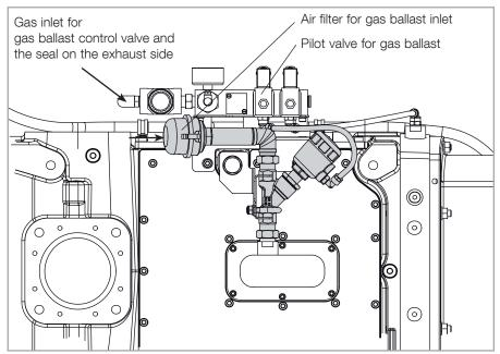
Fig. 3.7 Electropneumatic gas ballast valve (option)
