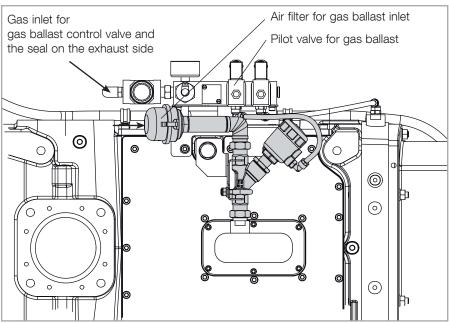
Fig. 4.6 Electropneumatic gas ballast valve (option)
