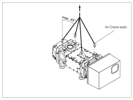
Fig. 2.1 Lifting the DRYVAC
