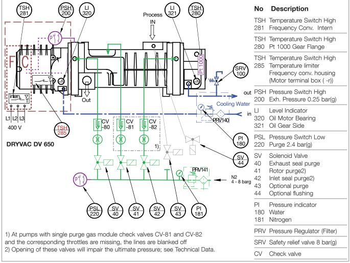
Fig. 3.8 Purge gas and switches schematic
