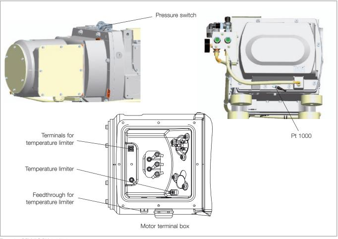
Fig. 3.15 DRYVAC DV 450/650-r sensors
