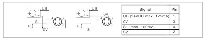
Fig. 3.10 Circuit diagram for the purge gas pressure switch
