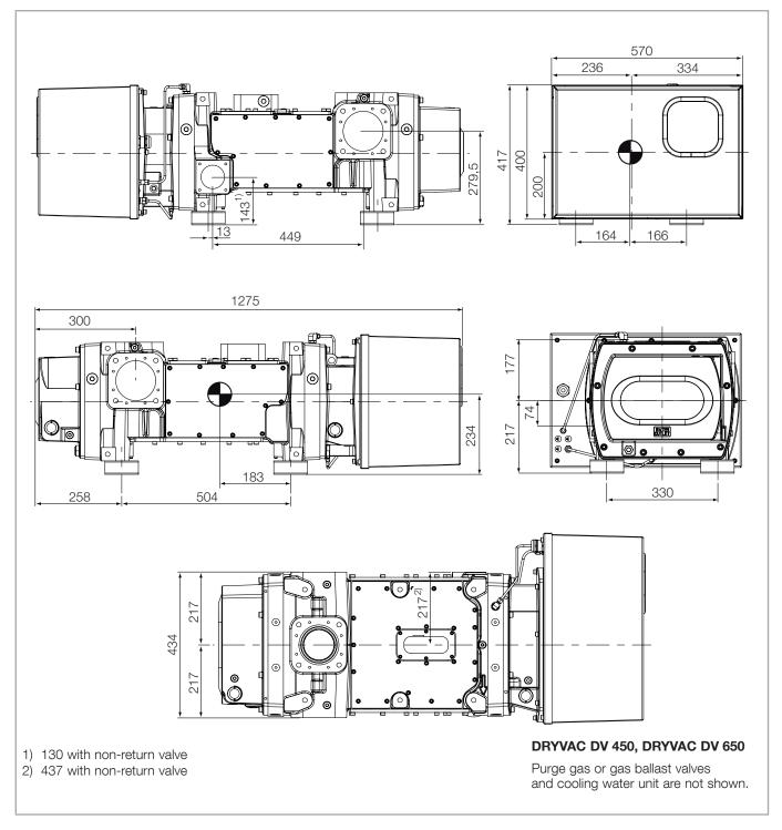
Fig. 1.6 Dimensional drawing, dimensions in mm
