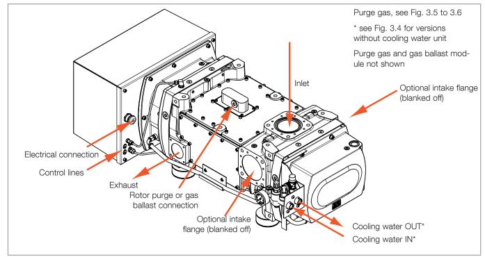
Fig. 3.1 Connections for the DRYVAC DV 450/650
