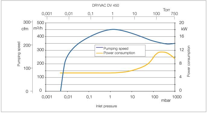
Fig. 1.3 Pumping speed curve
