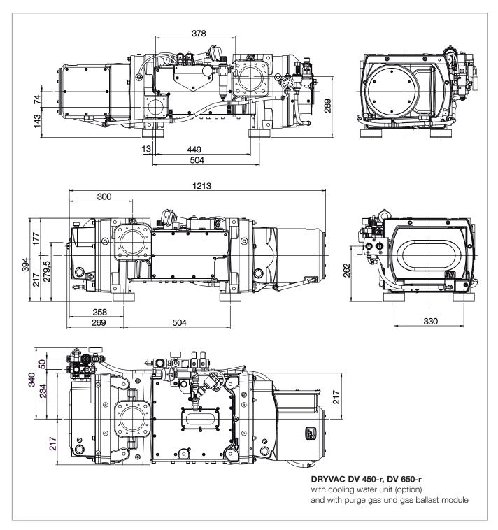
Fig. 1.7 Dimensional drawing, dimensions in mm
