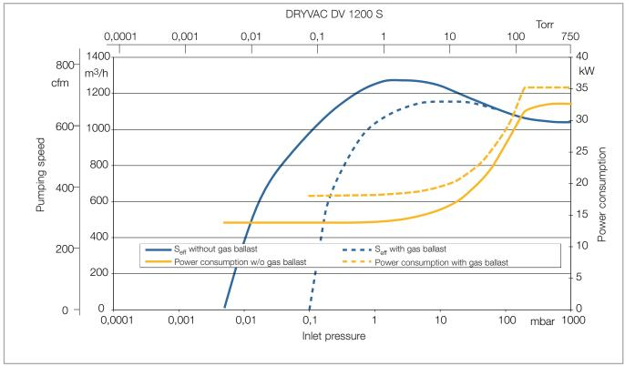
Fig. 1.5 Pumping speed curve
