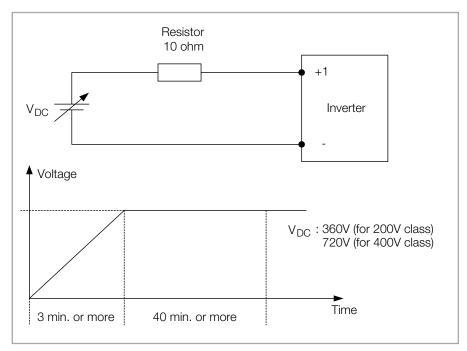
Fig. 2.2 Capacitor forming
