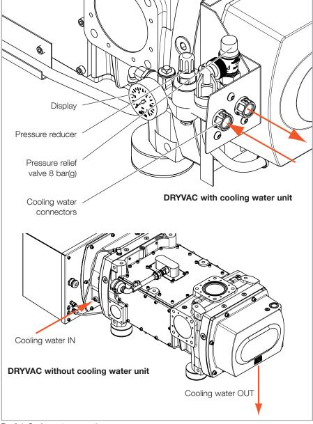
Fig. 3.4 Cooling water connection
