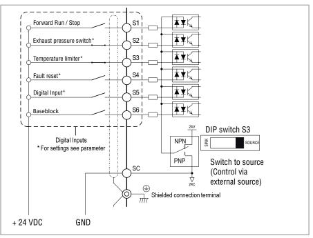
Option: Wiring with external power supply
