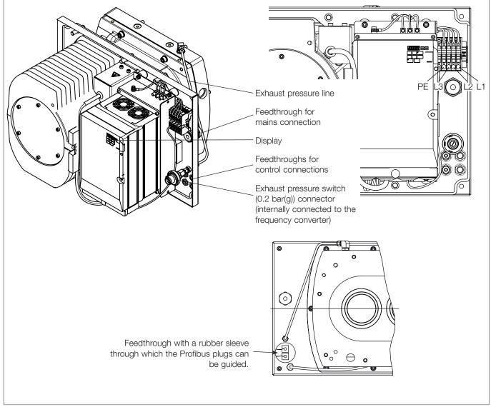
Fig. 3.12 Frequency converter without covers
