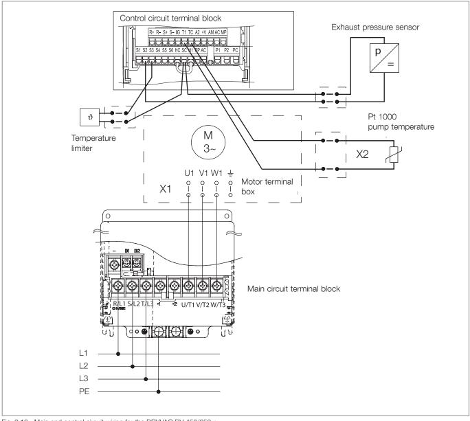
Fig. 3.16 Main and control circuit wiring for the DRYVAC DV 450/650-r
