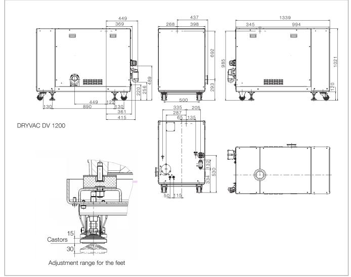
Fig. 1.8 Dimensional drawing, dimensions in mm
