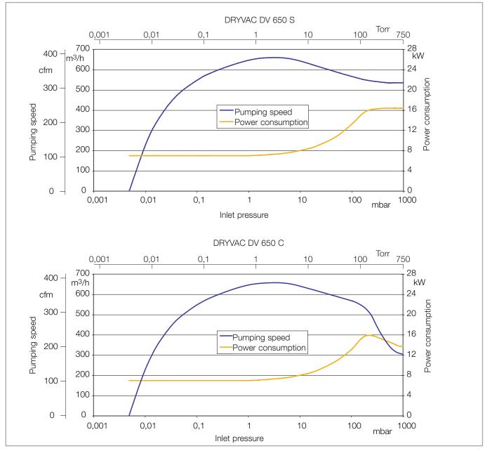
Fig. 1.4 Pumping speed curves
