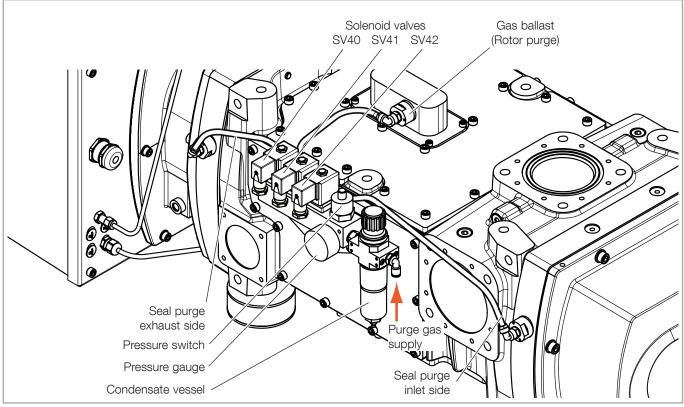
Fig. 3.5 Triple purge gas module (e.g. Part No. 112065V30-1)
