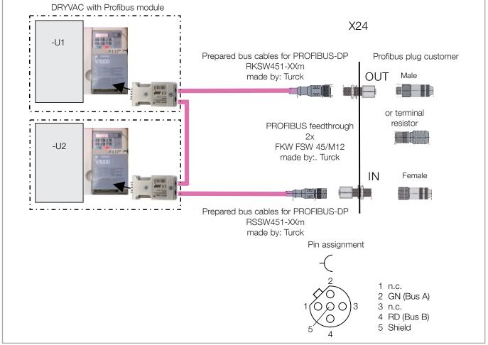
Fig. 3.20 Profibus connection
