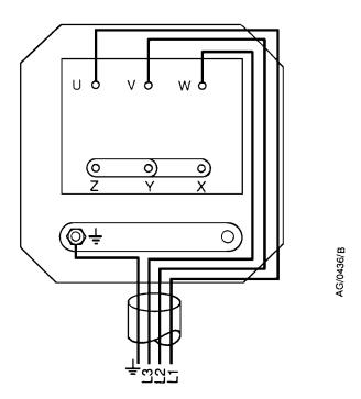
Figure 11 - ESDP30 motor terminal-box high-voltage configuration: 3-phase pumps
