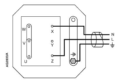
Figure 13 - ESDP30 motor terminal-box high-voltage configuration: 1-phase pumps
