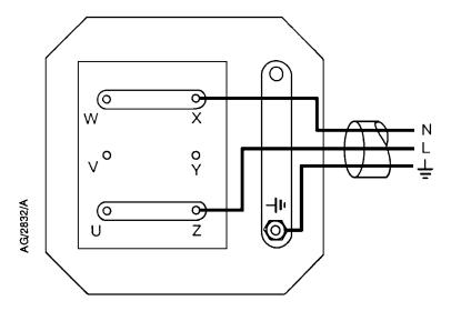
Figure 12 - ESDP30 motor terminal-box low-voltage configuration: 1-phase pumps
