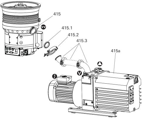
Fig. 10: Connecting the backing pump
