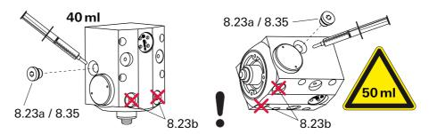
Fig. 9: Filling the operating fluid with vertical and horizontal installation orientation 8.23a Filler screw 8.35 O-ring
