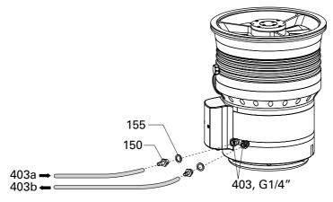
Fig. 15: Connecting the cooling water
