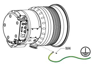
Fig. 11: Installing the earthing connection
