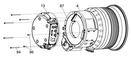
Fig. 20: Disassembly of the TC 1200
