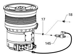
Fig. 13: Connecting the sealing gas valve
