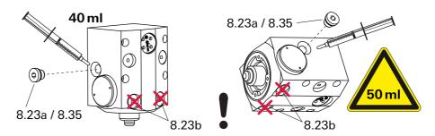
Fig. 19: Filling the operating fluid with vertical and horizontal installation orientation8.23a Filler screw8.35 O-ring
