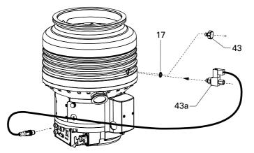
Fig. 12: Connecting the venting valve
