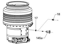
Fig. 13: Connecting the sealing gas throttle
