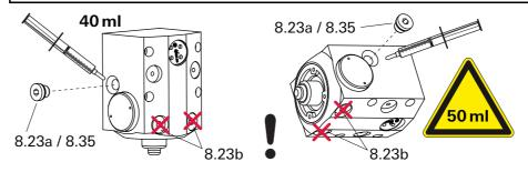
Fig. 9:Filling the operating fluid with vertical and horizontal installation orientation8.23aFiller screw8.35O-ring
