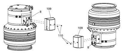
Fig. 17: Removing the protective cover of the operating fluid pump at standard and U-versions8Operating fluid pump109Protective cover110Allen head screw
