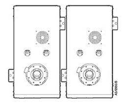
• The pumping system has provision to attach four seismic brackets however on the smaller systems, two brackets are capable of restraining the system during an earthquake. The smaller systems can therefore be secured as shown in Figure 6 for example, to reduce the effective system footprint if required. Refer to Section 7.3 to determine the correct seismic bracket kit for your system and for information about the systems which may be restrained with only two brackets.
