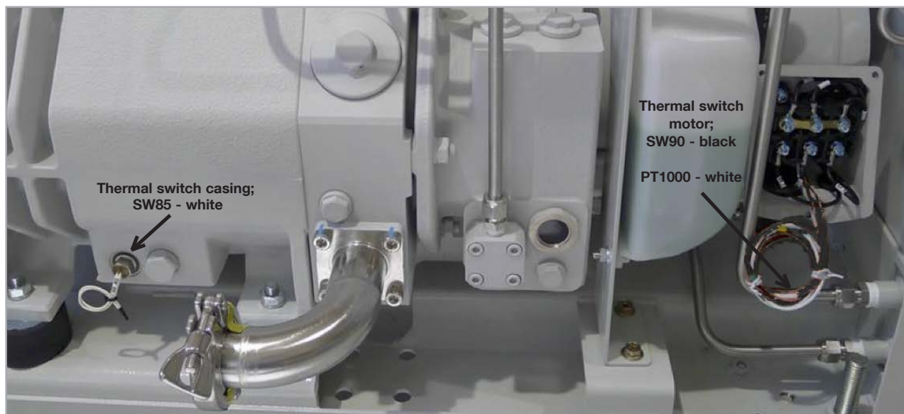
Fig. 3.3 Thermal switch positions
