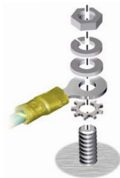
Figure 4-11: Ground Washer Stack Sequence
