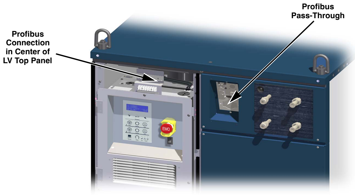
Figure 5-6: Profibus Pass-Through and Low Voltage Box Top Panel Connection
