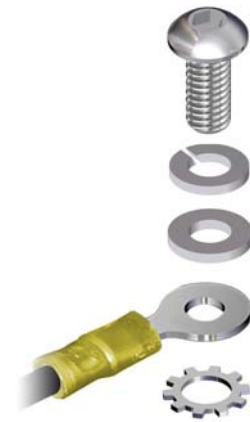
Figure 4-10: Terminal Washer Stack Sequence
