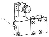
Press push-button (1): valve opens Release push-button (1): valve closes Figure 5-1
