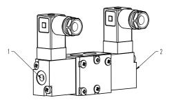
Press push-button (1): valve opens Press push -button (2): valve closes
