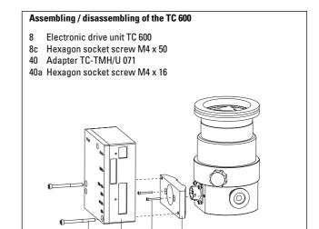
→ The adapter 40 must not be released for the replacement of the TC or following works.
