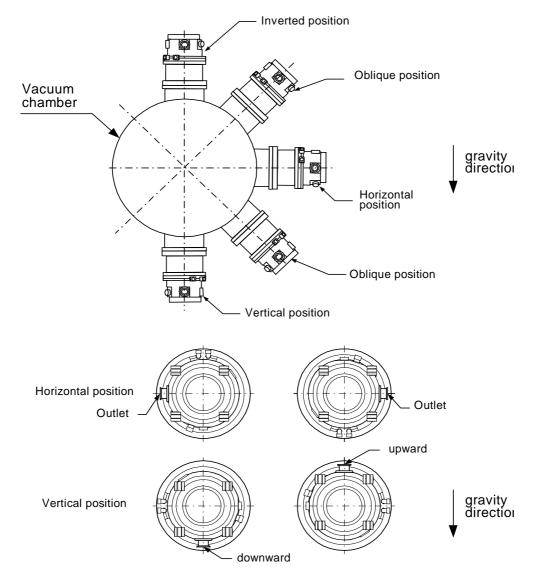
The outlet of the magnetic bearing turbomolecular pump should face horizontally or vertically when installing hotizontally.
