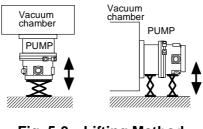
Fig. 5-3 Lifting Method
