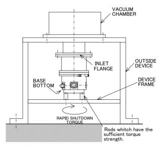
Fig. 5-5 Installation of Support Plate
