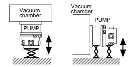
Fig. 8-1 Way to remove the pump
