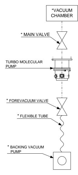
\* marks are not attached to this turbo molecular pump set.
