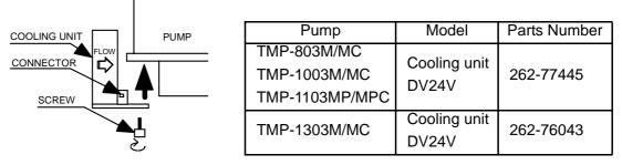
Fig. 1 How to Change the Cooling Fan Unit
