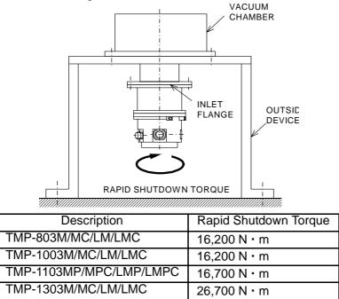
Fig. 5-2 Installation of Magnetic Bearing Turbo Molecular Pump
