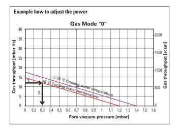
The following gas type characteristics lines enable you to adjust the power properly. At a cooling water temperature between 25 °C and 35 °C you have to draw your own gas type characteristics line.
