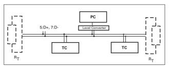
All units connected to the bus must have differing serial interface addresses (parameter 797). The group address of the TC 750 is 960.
