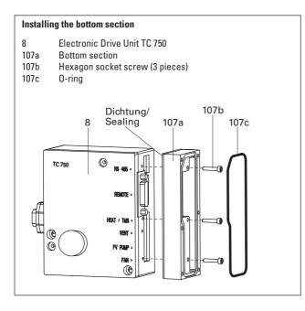
First pull the corresponding cables through the inserts with screwed cable glands and the cover 107d and insert the cables at the TC 750.
