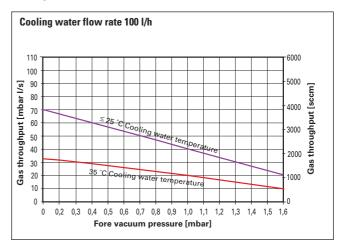
Gas type characteristics lines "Gas Mode 0"
