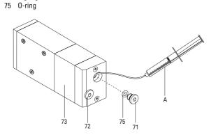
➡ Screw back in lubricant filler screw 71 with the 0-ring 75.
