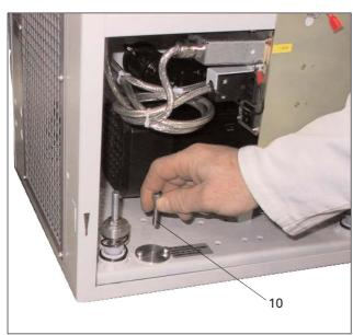
The transportation protection is now removed. The side panels can be re-fitted. Caution: Re-connect the earthing cable.
