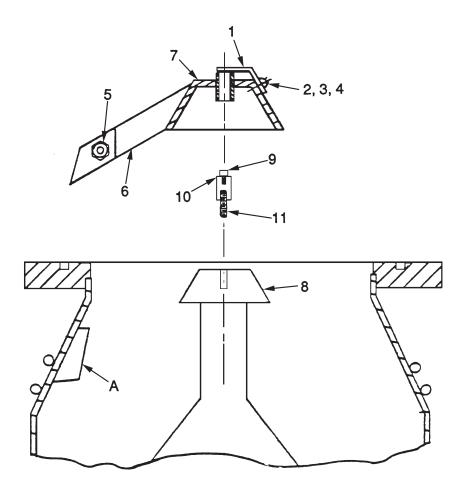
Figure 3-1 Cold Cap Removal/Installation
