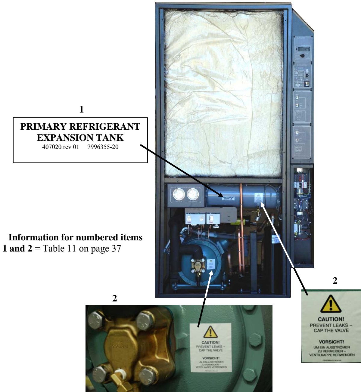
Figure 7. PFC 672 Internal Safety Labels, Front
