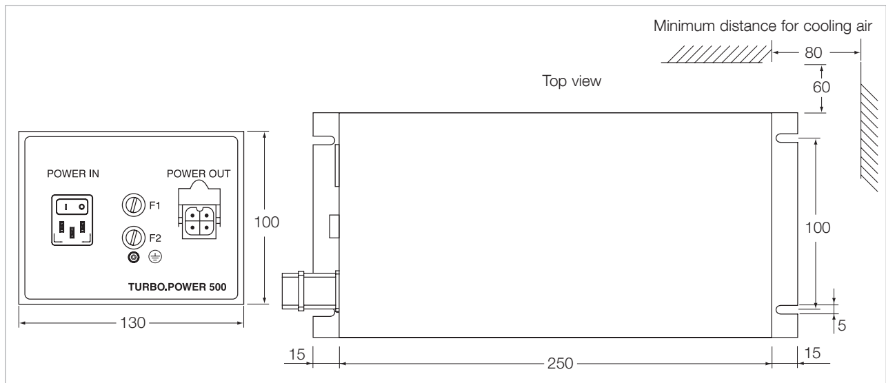
Fig. 1.12 Dimensional drawing for the power supply TURBO.POWER 500; dimensions in mm
