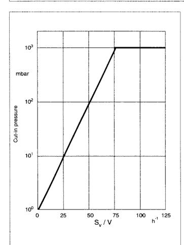
Sv = Pumping speed of the backing pump (m<sup>3</sup>·h·¹)V = Volume of the vessel (m³)
