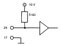
If pin 24 is not connected the normal operation speed is 500 Hz as default.
