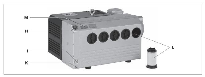
Fig. 7 Lubrication and removing oil
