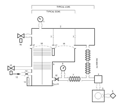
Figure 9 Typical pumping system with a nEXT pump
