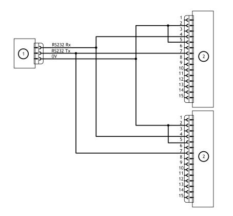
1. RS485 interface on control equipment 2. pump
