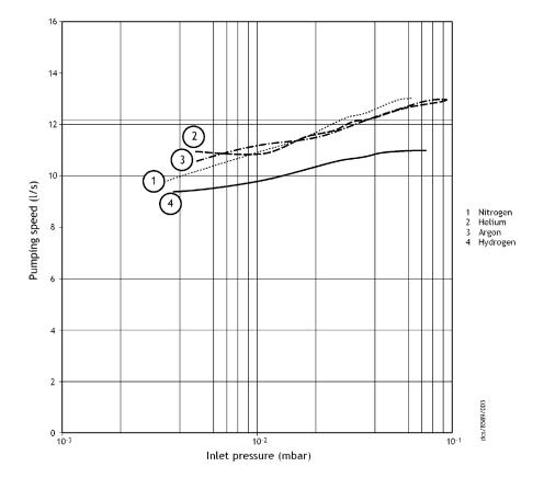
Figure 3 nEXT 200200 NW25 interstage port pumping speed
