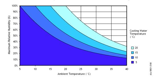
Figure 17 Maximum relative humidity to avoid condensation with water cooling
