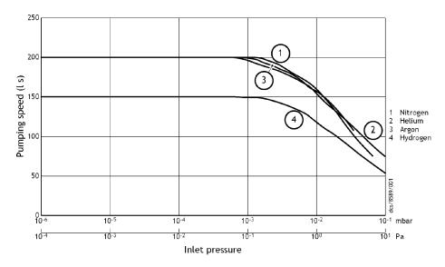
Figure 2 nEXT200200 side inlet performance curve
