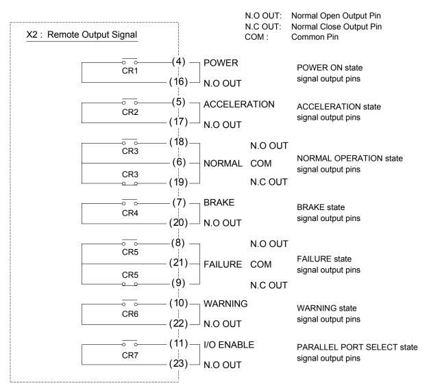
Figure 7.3 X2 REMOTE Output Signal Pins
