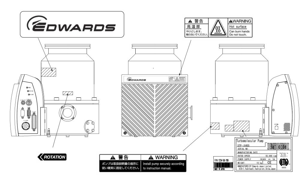
Figure 15.3 Label Affixing Positions for the STP Pump
