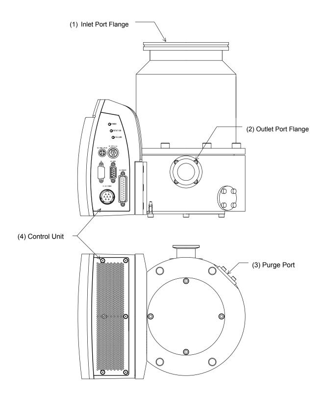
Figure 4.1 Configuration of the STP Pump
