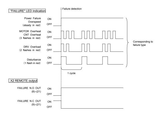
Figure 13.1 Failure Output
