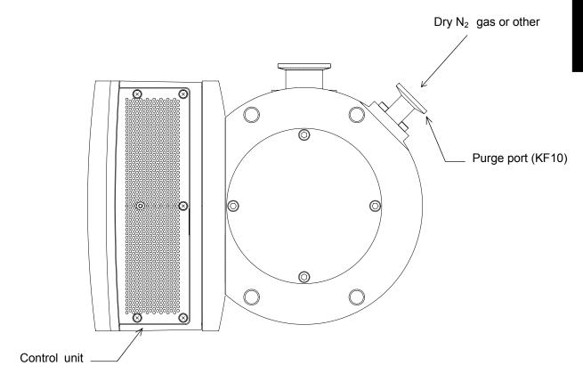
Figure 4.12 Connecting the Purge Port
