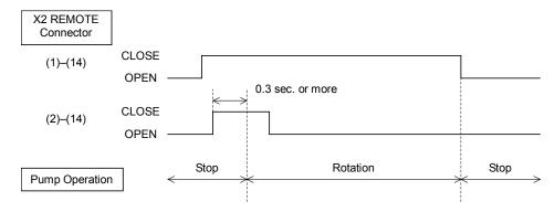
Figure 6.1 Pump Operation (Method 1)
