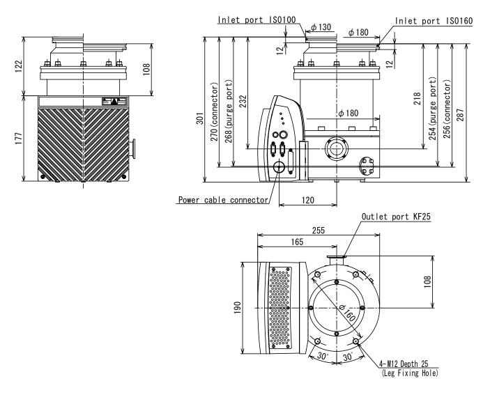
Figure 15.2 External Appearance of the STP Pump (STP-iXL455 series)
