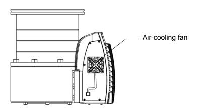
Figure 5.2 Air-cooling Unit U0-64
