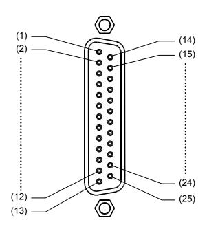
Figure 7.1 X2 REMOTE Pin Arrangement
