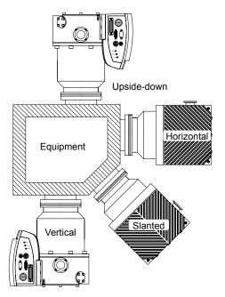
Figure 4.5 STP Pump Installation Positions
