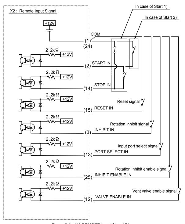
Figure 7.2 X2 REMOTE Input Signal Pins
