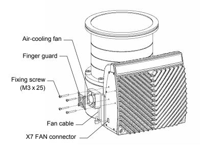
Figure 5.4 Installation Procedure for Air-cooling Unit U0-64
