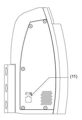
Figure 4.3 Control Unit (Rear panel)
