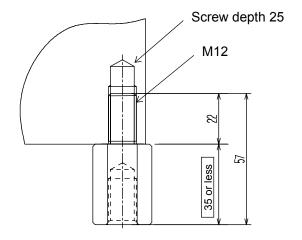
Figure 4.10 Recommended Leg for Securing Base
