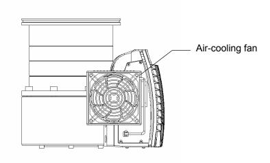
Figure 5.3 Air-cooling Unit U1-64
