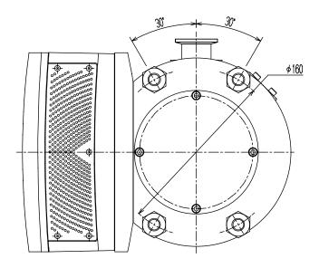
Figure 4.11 Position of the Screw Holes for Legs
