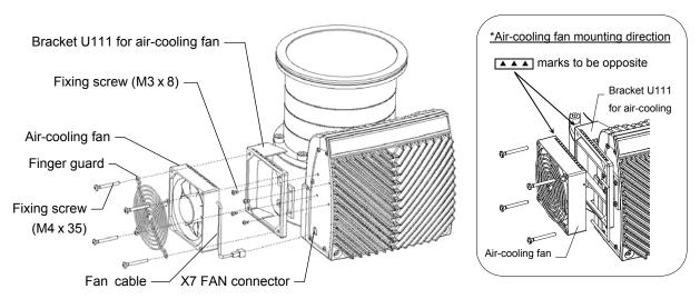
Figure 5.5 Installation Procedure for Air-cooling Unit U1-64
